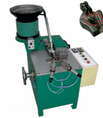
QLQ-012 Automatic Invisible Slider Body De-burr/Broaching Machine (Y shape, for cleaning tape slot, centre column)
