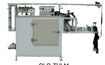
QLQ-THLM Automatic Metal Zipper Teeth-head Lacquer Machine (single cycle type available & double cycle type for choosing)
