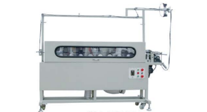
QLQ-10THPM Automatic Metal Zipper Teeth-head Intelligent All-around Polishing Machine (single side, 10 pcs wheels)
