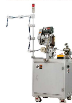
QLQ-BSM Automatic Metal Zipper Bottom Stop M/C (by brass bottom stop wire)
