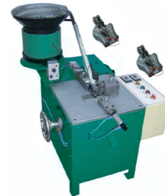
QLQ-011 Automatic Invisible Slider Body De-burr/Broaching Machine (I shape, for cleaning mouth height & width)
