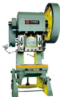
QLQ-NPM25 Automatic Pressing Machine (25T)
