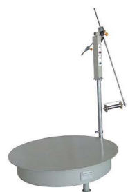
Wire Frame (horizontal system with transducer and electronic ruler)
