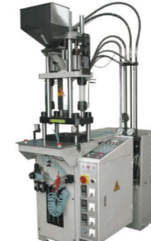
QLQ-SDIM-1 Semi-automatic Plastic Zipper Closed-end & Open-end Injection M/C (for zipper with/without slider)
