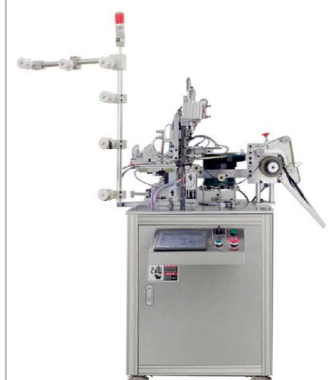
QLQ-MUTM Automatic Metal Zipper Top Stop M/C (by grain "U" shape top stop)
