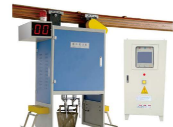
Automatic Zinc Material Feeding System
