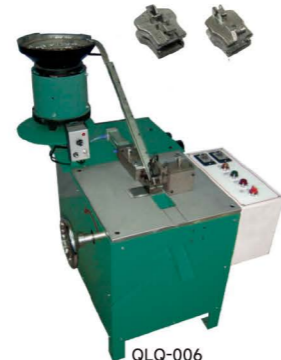
QLQ-006 Automatic Slider Body De-burr/Broaching Machine (for 1 pc of slider body)
