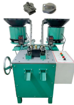
QLQ-061 Automatic Slider Body De-burr/ Broaching Machine (for 2 pcs of slider bodies)
