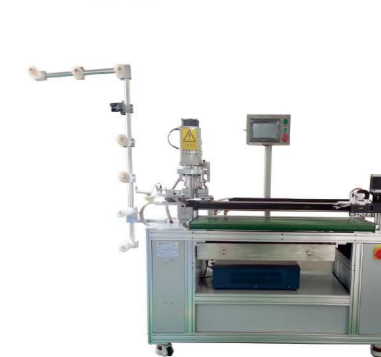
QLQ-OCM-4 Automatic Nylon Zipper Ultrasonic Open-end Cutting M/C (with labour hand)
