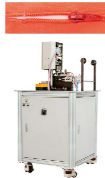
QLQ-SNUTM Semi-automatic Nylon Zipper Ultrasonic "U" Shape Top Stop M/C (by transparent top stop wire)
